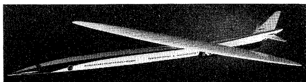
Fig. 3 Oblique-wing transonic transport (concept of R.T. Jones).
